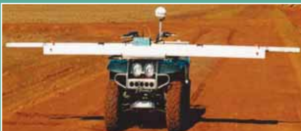
Figure 1 The EM31 mounted in the vertical dipole surveying position on a non-conductive frame and connected to a differential GPS on a 4-wheel motor bike
