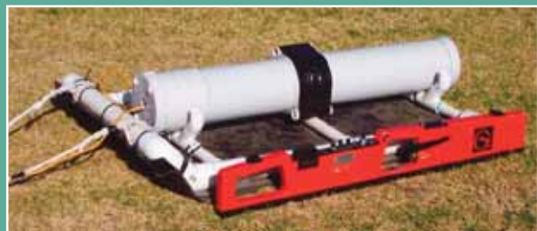
Figure 2 EM38 in the vertical dipole position, next to a non-conductive sled into which it is placed then towed behind a 4-wheel motor bike to survey fields
