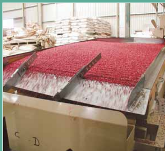
Figure 2 First grade yield is beans graded over a 4 mm (10/64") slot screen and usually represents 75–85% of the total yield and about 95% of the total income
