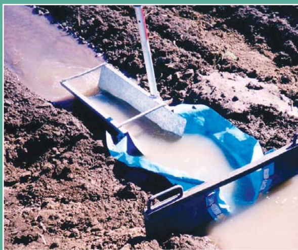
Figure 1 The Irrimate™ in-field surface irrigation evaluation service provides irrigators with a means of assessing surface irrigation performance and in conjunction with integrated software, identifies possible management changes to improve efficiency. The Irrimate monitoring package contains a siphon flow meter (left), water advance sensors, an in-furrow downstream flume (right) and computer software.
