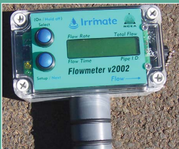
Figure 1 The Irrimate™ in-field surface irrigation evaluation service provides irrigators with a means of assessing surface irrigation performance and in conjunction with integrated software, identifies possible management changes to improve efficiency. The Irrimate monitoring package contains a siphon flow meter (left), water advance sensors, an in-furrow downstream flume (right) and computer software.
