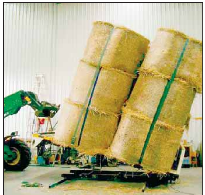
Figure 1: A tilt test in progress. Photo AFIA.
