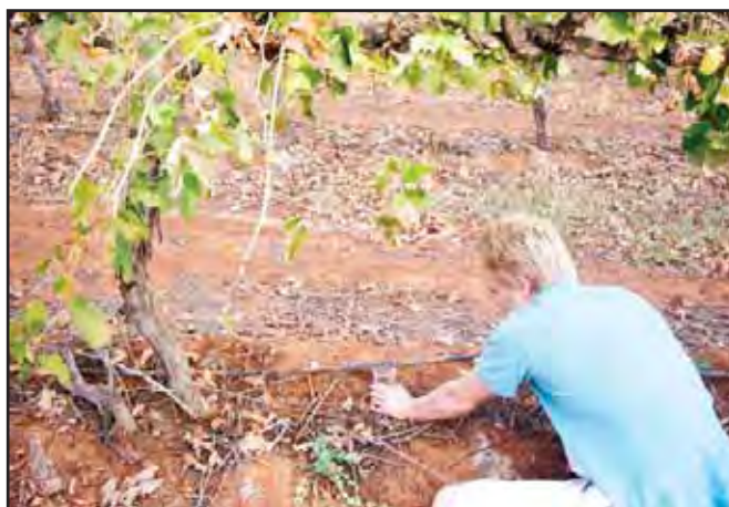
Figure 1: Measuring drip emitter rates in a vineyard using a 'catch can'
