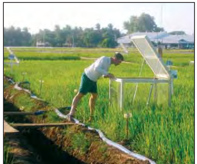
Figure 3: The author risking decapitation by an automated gas chamber at IRRI. The chambers close and sample the air above the crop for greenhouse gases.
