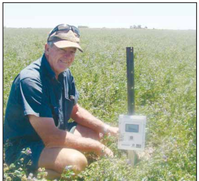
Figure 1. Soil moisture levels can be monitored using gypsum blocks to better understand likely crop requirements for water.
