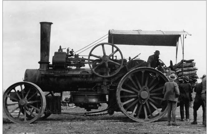
McCaughey's steam engine was used to drag rippers to break up the ground for farming. Photo: Mr Correy, supplied by his daughter Mrs Carrig.
