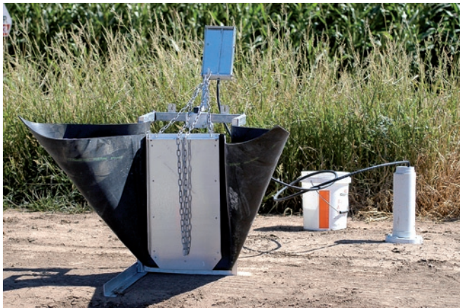
Figure 2. A "Padman Stop" with a pneumatic controller for opening and closing the stop automatically. The controller is connected to an air tube and responds to a relative level of water in the tube.
