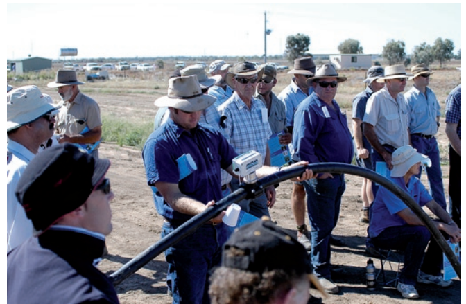
Figure 3. Irrimate siphon meter used for performing in-field evaluations of water behaviour in furrow irrigation layouts.
