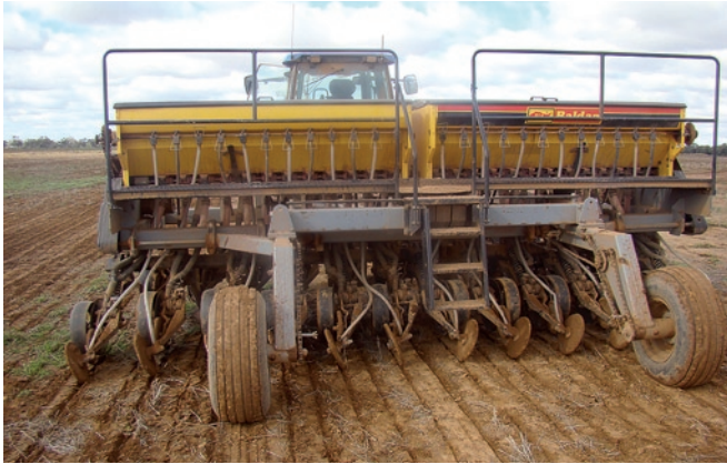
Figure 1. A single disc seeder is central to managing large stubble loads in a direct drilling program at Forbes. Row widths have been widened to fit in with bay widths and allow more stubble flow.
