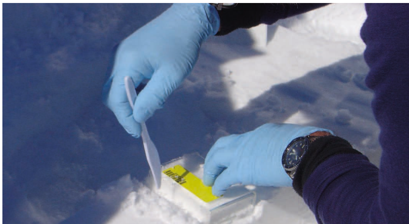
More than 2000 samples of snow, soil and water are collected each year to measure concentrations of the seeder and tracer agents in terrestrial and aquatic environments. Six years of data provides compelling evidence that cloud seeding has not had any significant adverse environmental impact.
