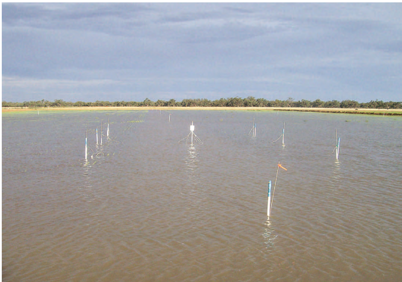
Water depth loggers and soil waterlogging sensors in one of the bays monitored during the study. Although the bay only took four hours to fill, water was on the bay for 44 hours and it took another 59 hours for the soil to drain. So oxygen levels in the soil were decreasing for over 100 hours.
